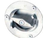
The grinding mechanism is provided at the suction port of the pump. Flown in suspended solids are cut into small pieces and pumped out. This mechanism eliminates a fear of clogging in small diameter pipes.
