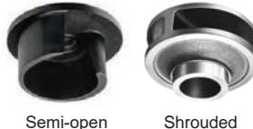
The impeller is semi-open or shrouded type with single or two vanes. It has a wide channel extending from inlet to exit, which allows the pump to pass the solid matters from inflow to discharge with minimal blockage.
